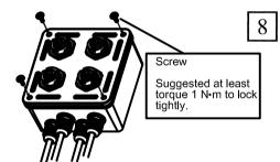
Attach the frame on the box using screws until snug. Do not over tighten! insert.
