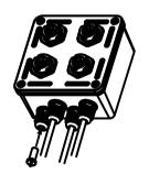
Insert the filler into any empty waterproof insert to seal the box. The installation is now complete. (Filler goes with 2 port upward box.)
