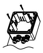
Secure the box to the wall with three screws.
